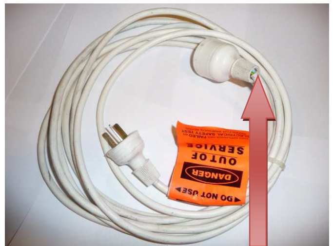
"light duty" extension lead – blue & green wires showing
