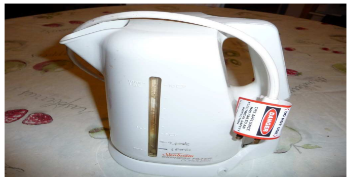
FAILED Kettle - earth resistance exceeded the safety limit
