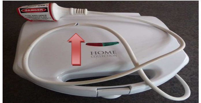
FAILED - Sandwich Toaster has a melted lead
