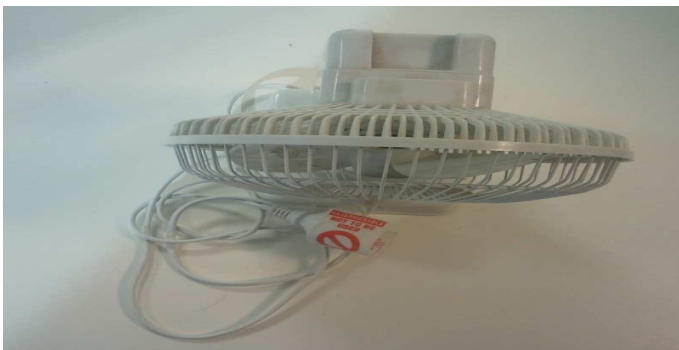
FAILED Desk Fan - slow speed switch not working
