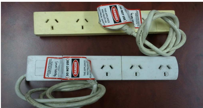
FAILED – Power boards have broken parts inside
