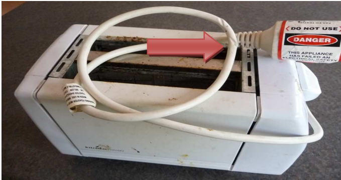
FAILED - Toaster has a melted lead
