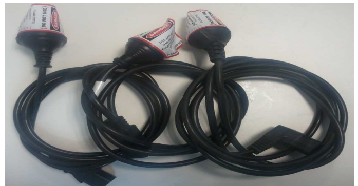
FAILED an earth bond test - Computer IEC Power Leads
