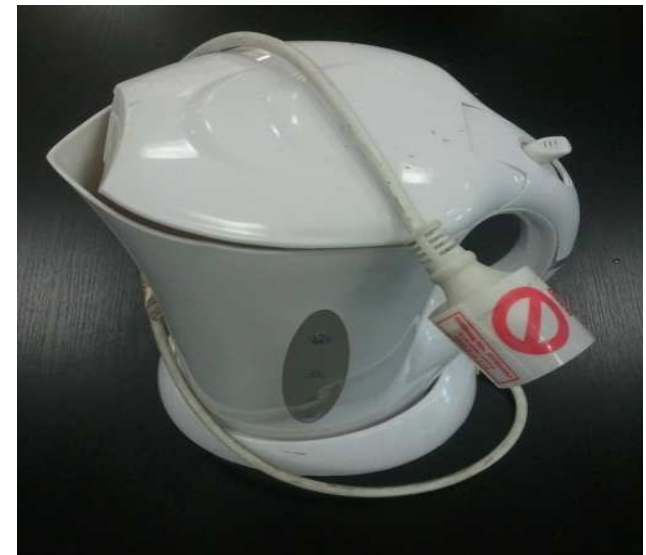
* Tag 047 Kettle FAILED - Does not switch off
