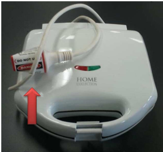
* Tag 049 FAILED - has a damaged lead
