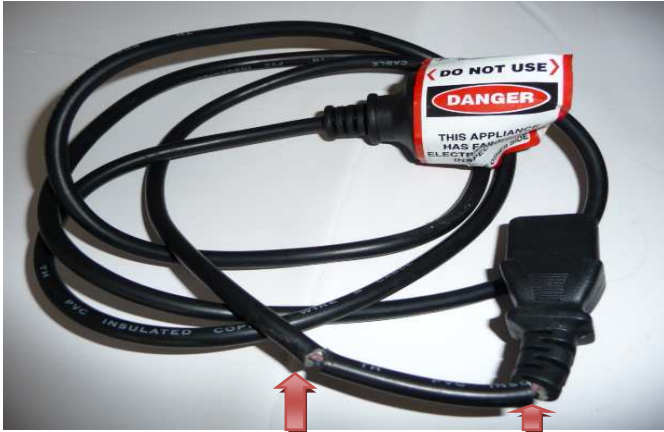
Computer power lead with cuts
