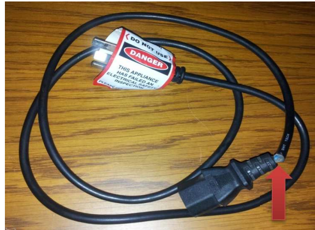
* Tag 005 damaged IEC power lead
