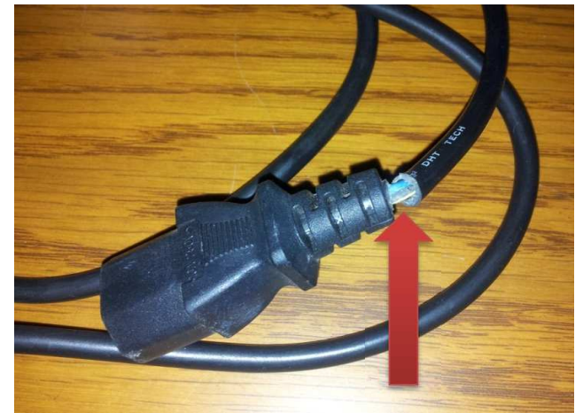
* Tag 005 damaged IEC power lead
