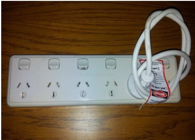
* Tag 001 FAILED - loose insides
