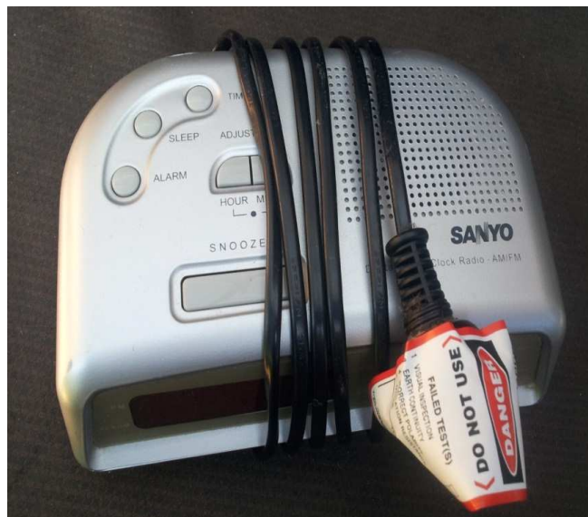
* Tag 043 FAILED - squashed lead
