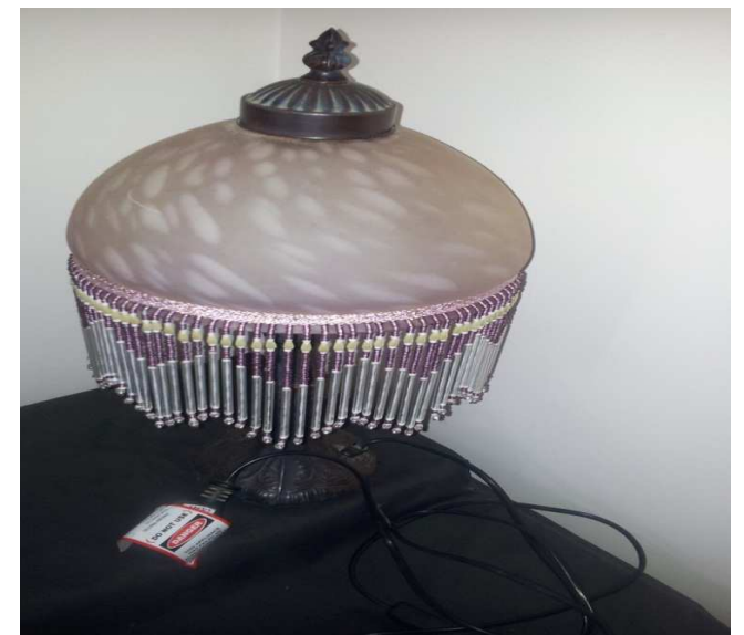
* Tag 055 FAILED - squashed lead
