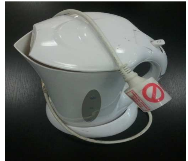
* Tag 047 Kettle FAILED - Does not switch off
