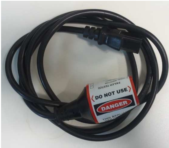
* Tag 004 - PC IEC Lead FAILED Earth Bond Test
