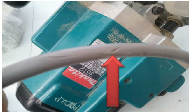
*Tag WS005 Had a new plug fitted and passed a re-test
