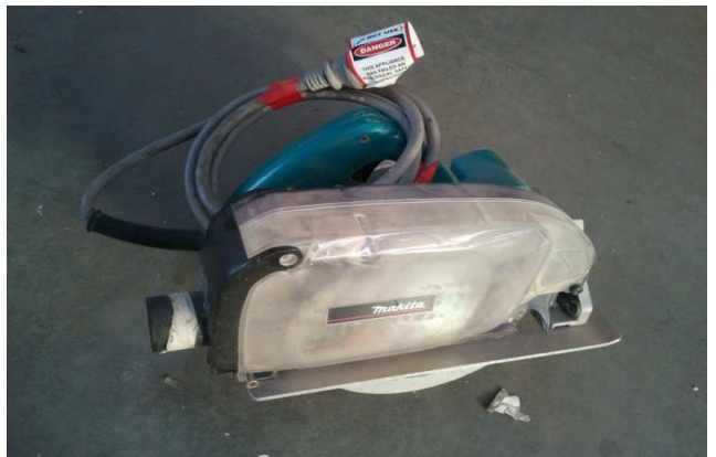
* Tag WS022 FAILED - Damaged lead
