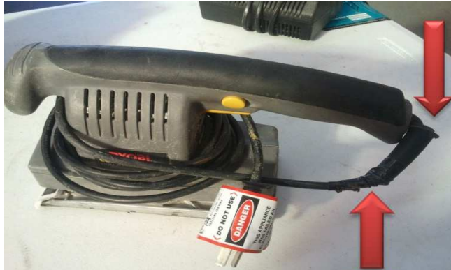
* Tag WS013 FAILED - Damaged Lead & Grommet
