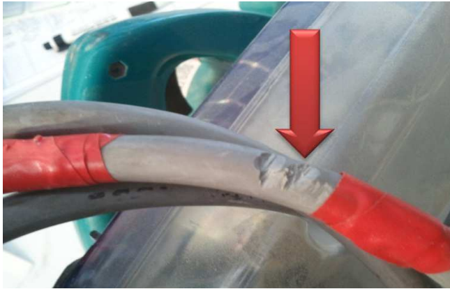
* Tag WS022 FAILED - Damaged lead
