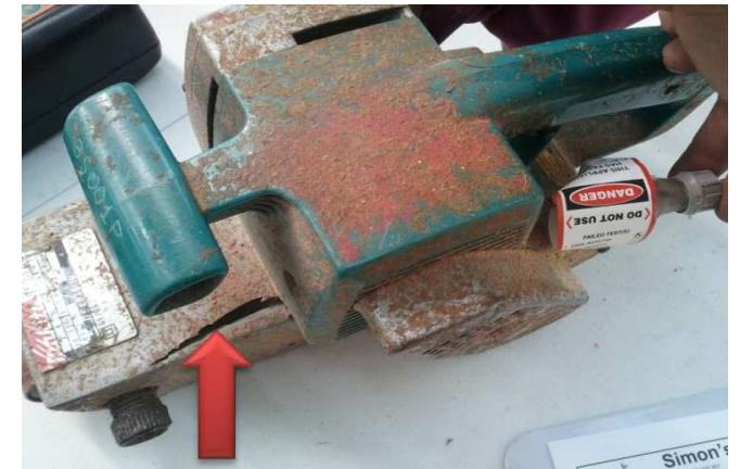
* Tag WS004 FAILED - Damaged Body
