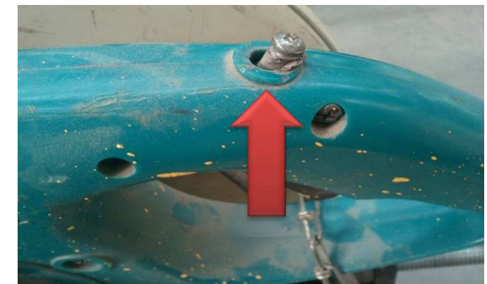
* Tag WS041 FAILED a Visual Inspection - Has a screw locking the top safety switch on
