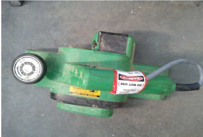
* Tag WS001 FAILED Lead and a Insulation Leakage Test
