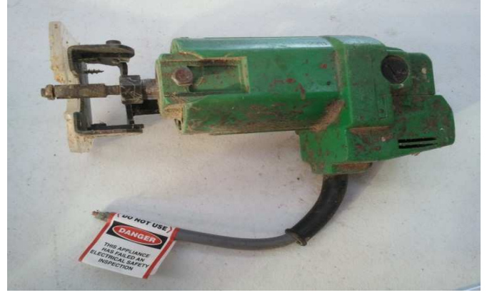
* Tag WS024 FAILED - Damaged Lead (short) & Body
